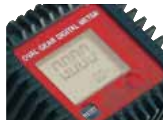
Multifunction display. 5 digit partial. Total. Resettable total and calibration available. Low battery icon.
